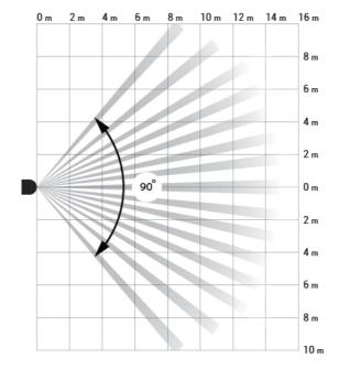
Make sure that no obstacles block the view of the detector. Note that MotionCam Outdoor does not detect movement behind the glass. Therefore, do not install the detector in locations where an open window or door can obstruct its view.
