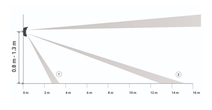
The detection distance is adjusted using the **Detection Distance** scrollbar on the rear panel of the detector. When choosing the installation location, consider the maximum detection range of the detector. It depends on the sensitivity, the position of the Detection Distance scrollbar, the type and speed of the person's movement (running, walking), and the ambient temperature.
