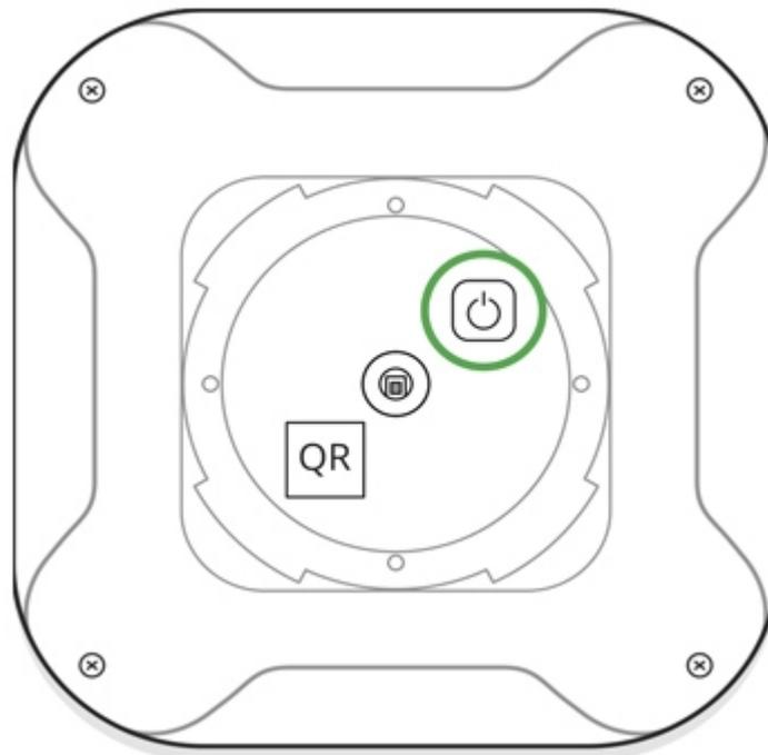
To make sure that the detector is on, press the on/off button – the logo will light up red for a second.
